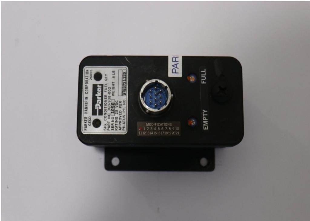
8. **Brief Description:**The fuel quantity detector system for each wing tank has three capacitance-type tank sensors and a fuel quantity amplifier. The anodized aluminum sensors, protected by polyurethane, are installed vertically and attached by spring clips to the nose ribs 12, 16 and 19. The sensors are connected in parallel and may be considered, electrically, one unit.
